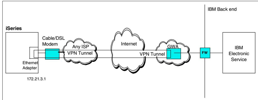
Figure 118. Direct cable modem network configuration
