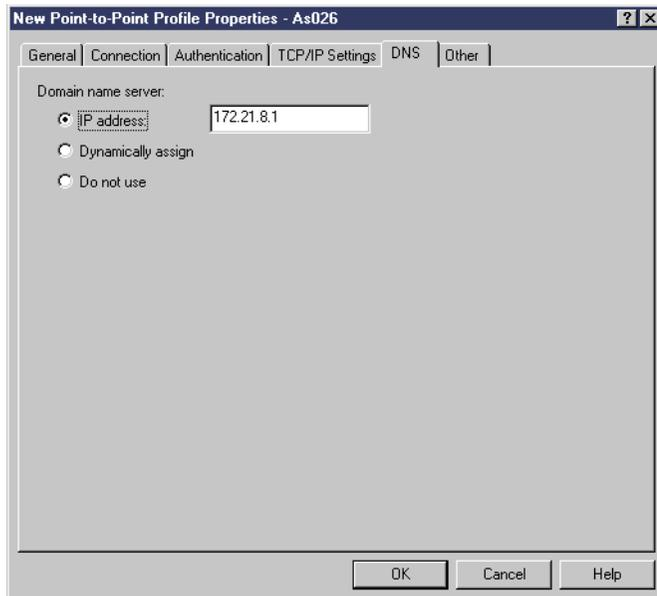
Figure 80. New Point-to-Point Profile Properties: DNS tab
