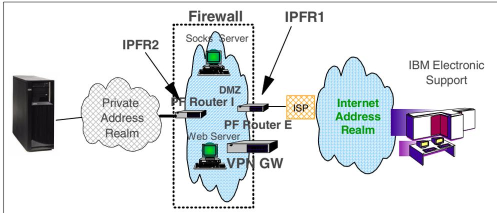
Figure 146. Merged interior router and stand-alone VPN secure gateway configuration
