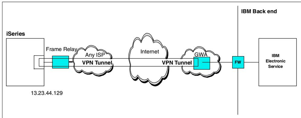
Figure 95. Frame relay network configuration
