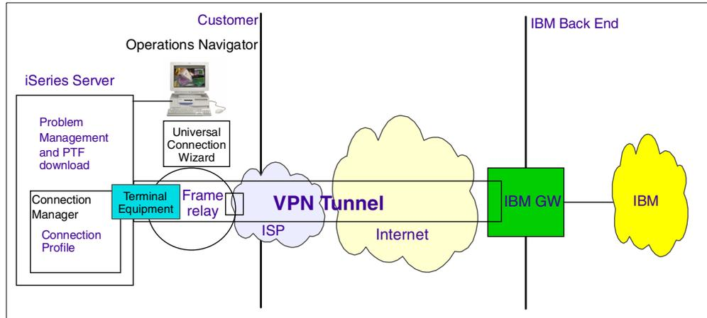
Figure 94. Network configuration using frame relay
