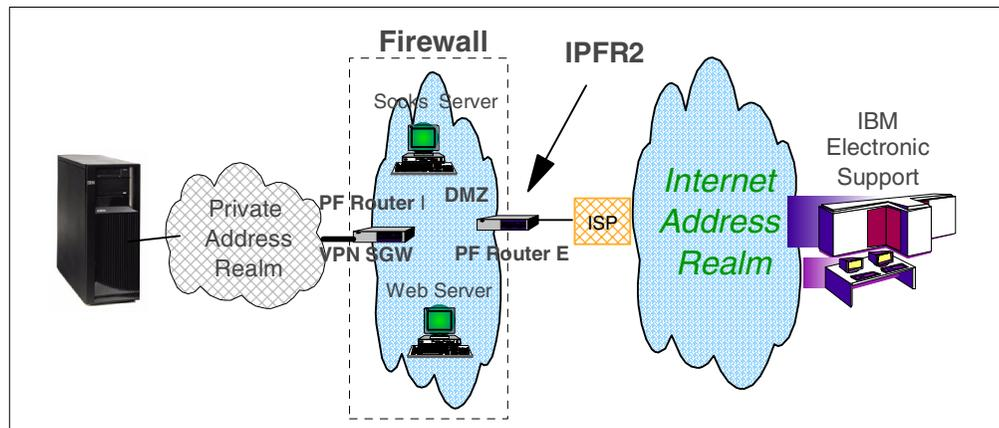
Figure 143. Merged interior router with VPN secure gateway configuration
