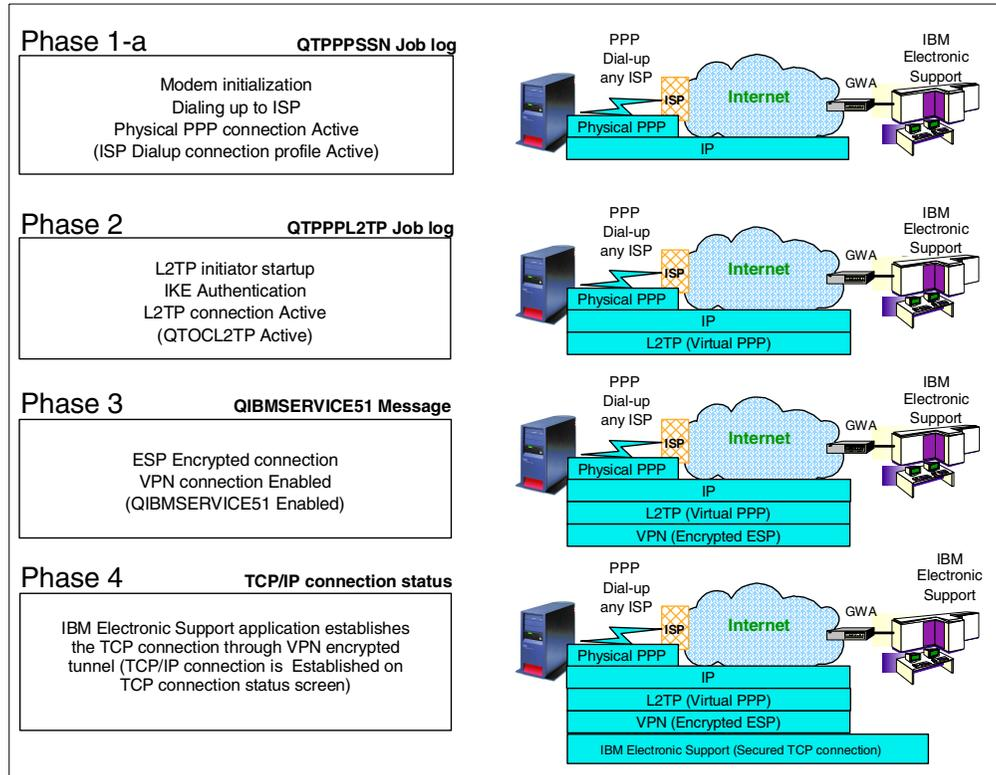
Figure 176. IBM Electronic Support VPN connection overview: Dial-up any ISP case
