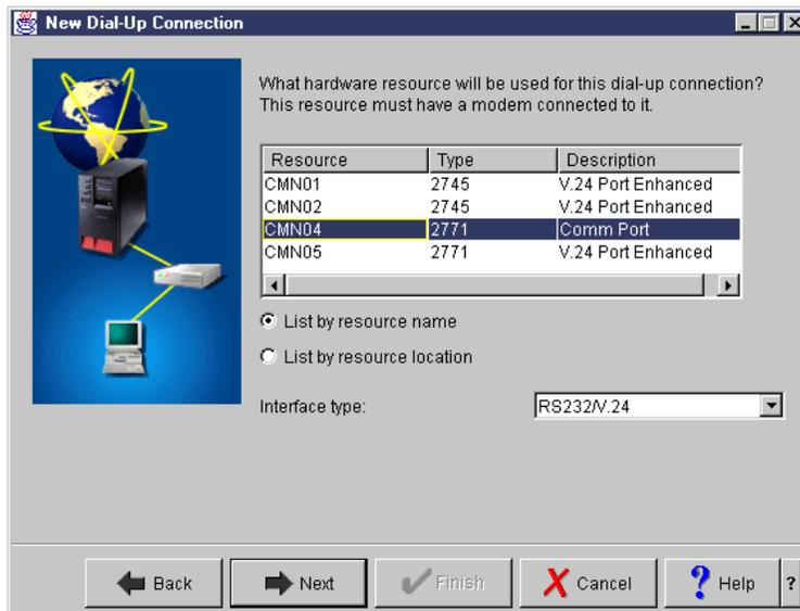
Figure 47. Selecting hardware resources: F/C2771 internal modem
