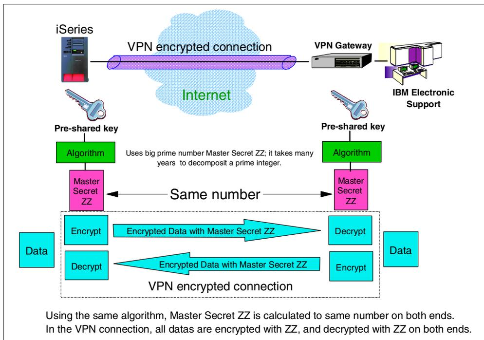
Figure 91. IBM Electronic Support connection using VPN
