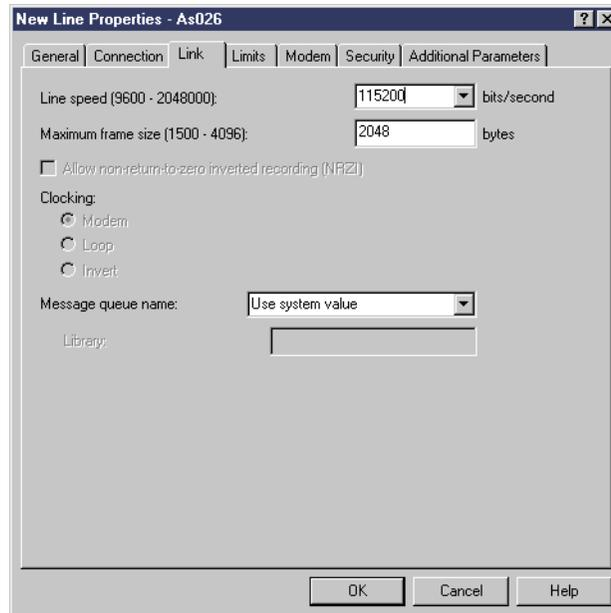
Figure 73. New Line Properties: Link tab
