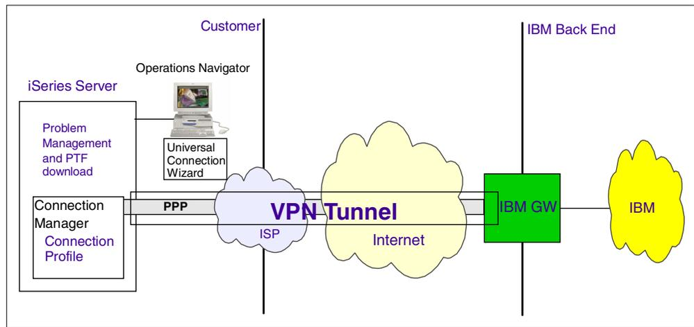
Figure 42. Network configuration of PPP dial-up to any ISP
