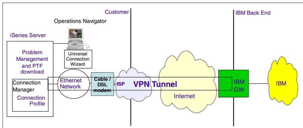
Figure 117. Direct cable modem/DSL modem network configuration
