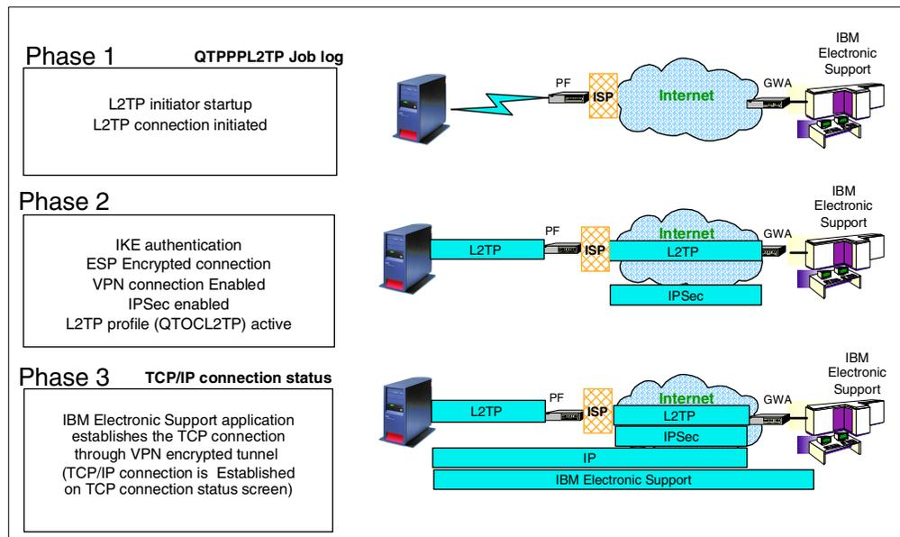
Figure 191. Phases of a multi-hop connection
