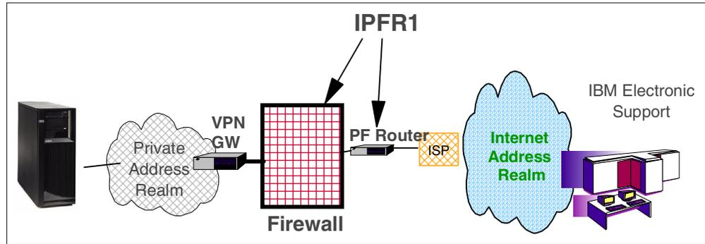
Figure 145. Standalone VPN gateway with Packet Filter router
